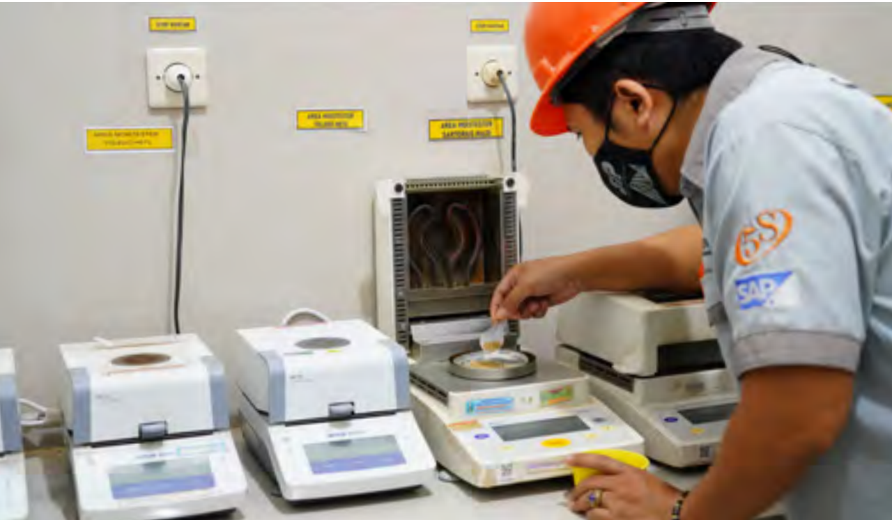
Moisture testing of aquafeed at Japfa Aquafeed Lab in Banyuwangi, Indonesia
