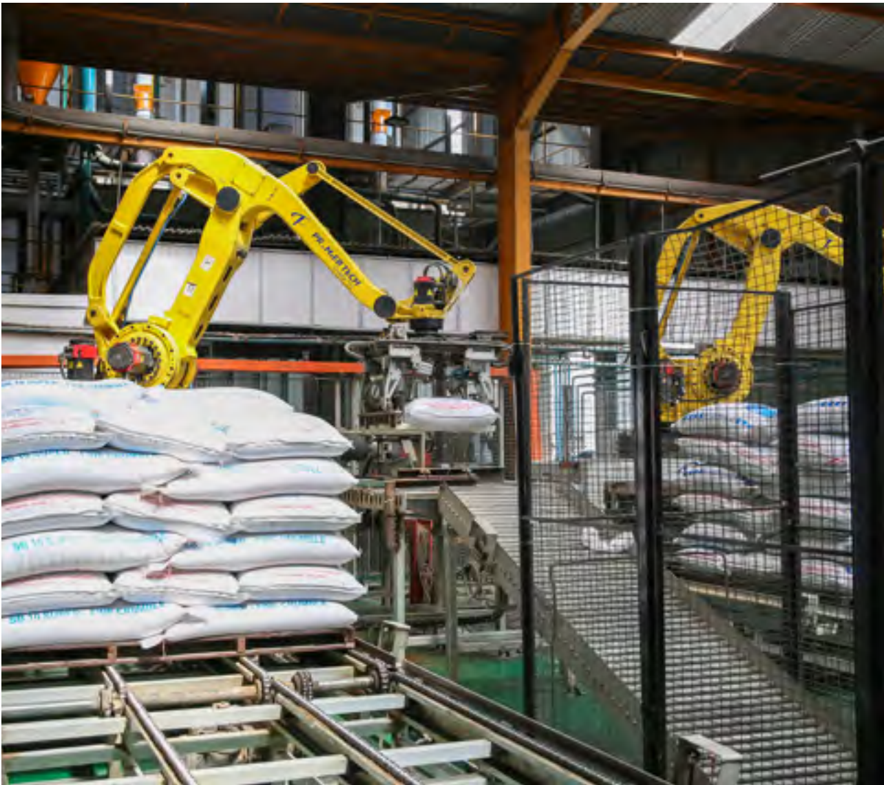
Robot palletising system in PT Japfa Tbk feedmill production line: Japfa continuously upgrades systems and machinery in our operations
